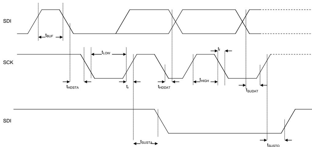
Figure 14: I<sup>2</sup>C timing diagram
