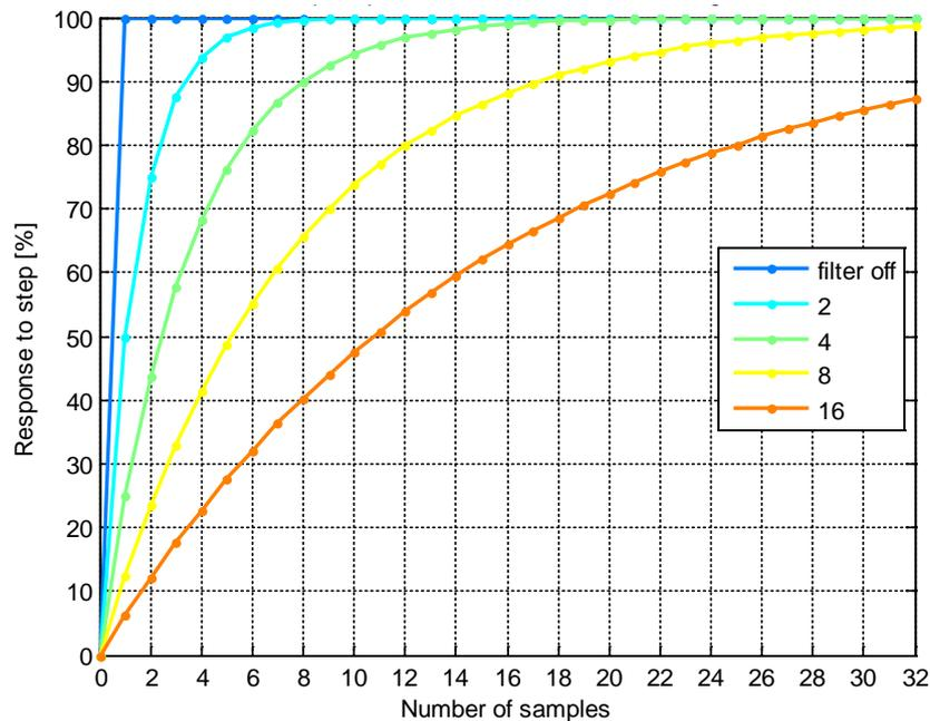
Figure 7: Step response at different IIR filter settings
