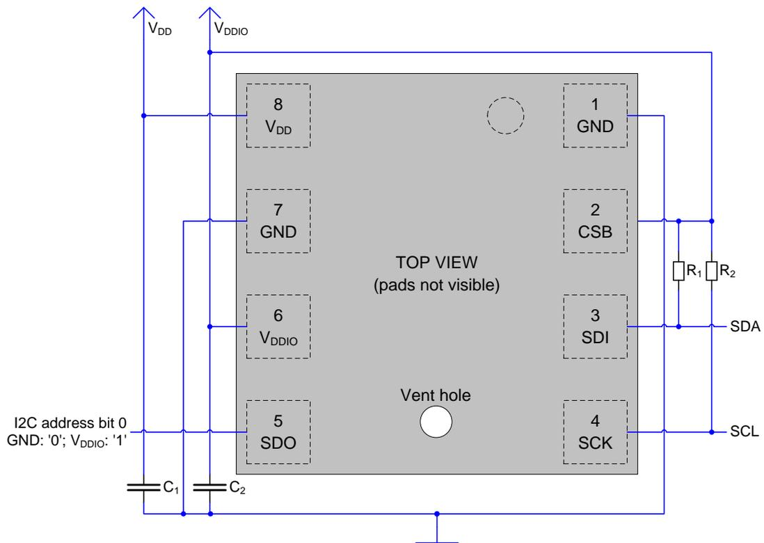
Figure 17: I<sup>2</sup>C connection diagram
