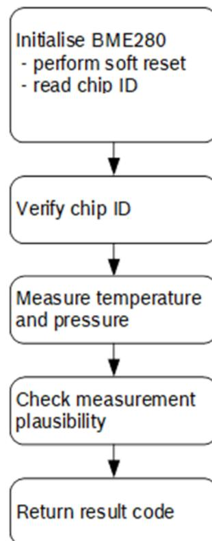
Figure 25: Self-test flow chart
