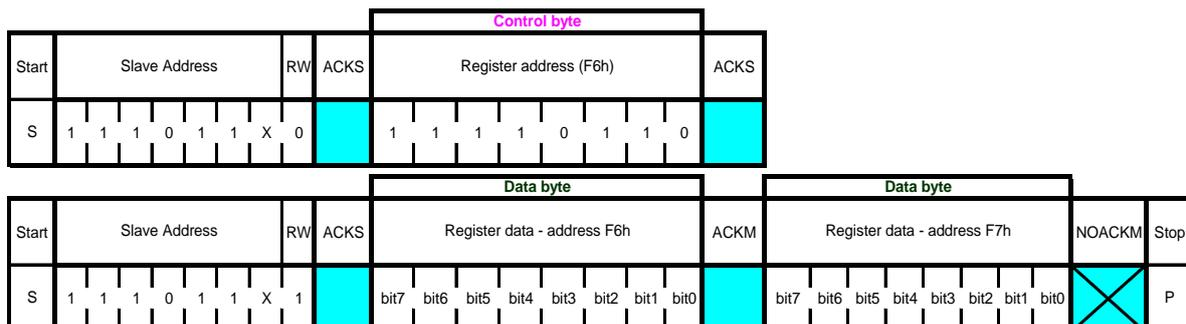
Figure 10: I<sup>2</sup>C multiple byte read
